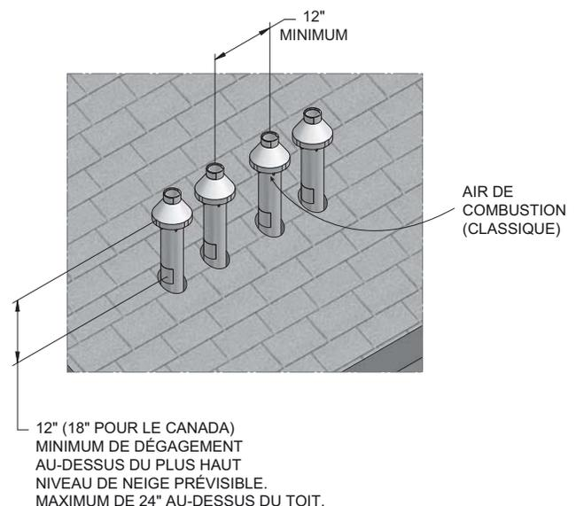
12" (18" POUR LE CANADA) MINIMUM DE DÉGAGEMENT AU-DESSUS DU PLUS HAUT NIVEAU DE NEIGE PRÉVISIBLE. MAXIMUM DE 24" AU-DESSUS DU TOIT.
